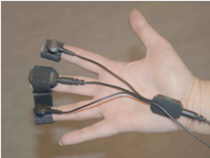
Fig. 03. Measurement of the electrodermal activity (index and ring fingers), BVP (middle finger).
