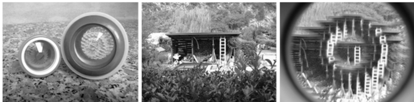
Fig. 18. The “magic eye” uses the law of refraction. a) It is like a rosette with several surfaces cut under different angles. An object (shelter of the neighbor, b) is multiplied (c) into as many images as the number of separate surfaces in the “eye”.
