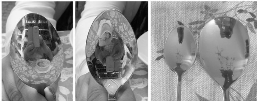
Fig. 11. Spoons as mirrors: a) a convex surface gives non-inverted image, b) a concave mirror – an inverted image (hand of Ula Kordowska, a constant distant from the spoon was kept). c) In Korea two types of spoons are used at table: the smaller one gives a smaller image (a concave surface, image of the rose on the table that was above the spoon).
