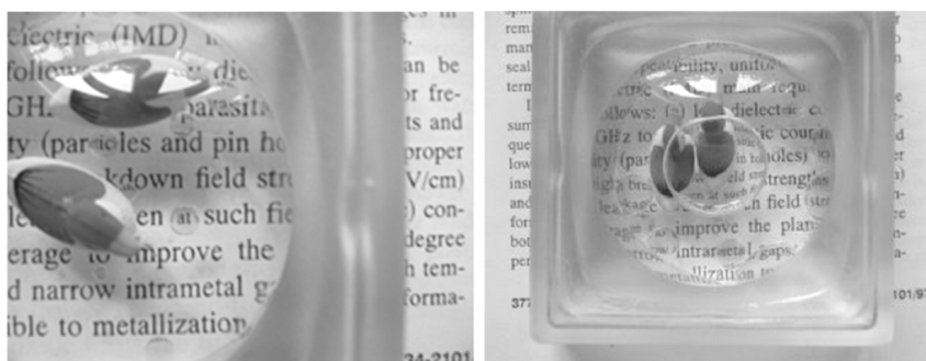
Fig. 27. A toy ash-tray filled with water: the central convex part acts as a magnifying lens, spherical-like air bubbles in water act as a de-magnifying lens. Objects and photo GK.
