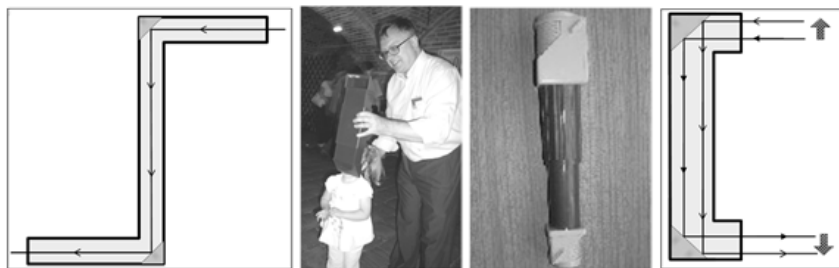
Fig.2. Fun with periscope: a) a scheme of a correct construction and b) its application – how to see the world like an adult (“Fiat Lux” exhibition in Toruń, 2007); c) a toy periscope that allows to rotate the upper part: the images rotate with turning the periscope; d) a scheme of a “wrongly” mounted periscope.
