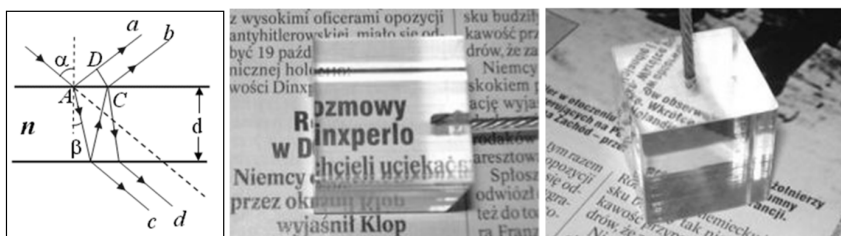
Fig. 16. (a) Light passing through a flat piece of glass (or a cube) is deviated twice. As a result, rays entering parallel exit also parallel. b) In this manner, the object below seems to be shifted. c) If the cube is rotated, not only the shifted image is seen but also a reflection of the object on the inner face of cube.
