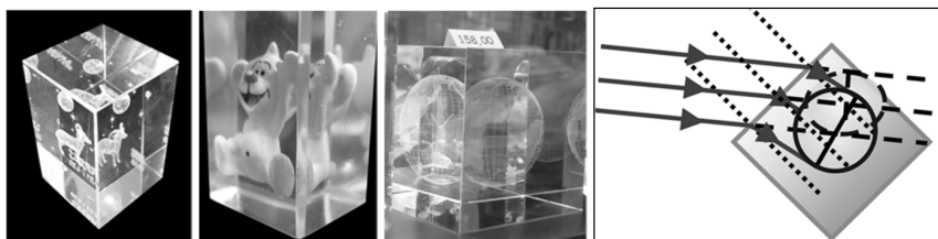
Fig. 17. Fun with refraction: seeing objects from three sides at the same time – objects are printed inside glass cubes and what is seen are projections of three perspectives onto three perpendicular surfaces (a-c). As shown at c, i.e. an image of the sphere, these projections are rescaled in the directions of observation, as shown on the scheme d).
